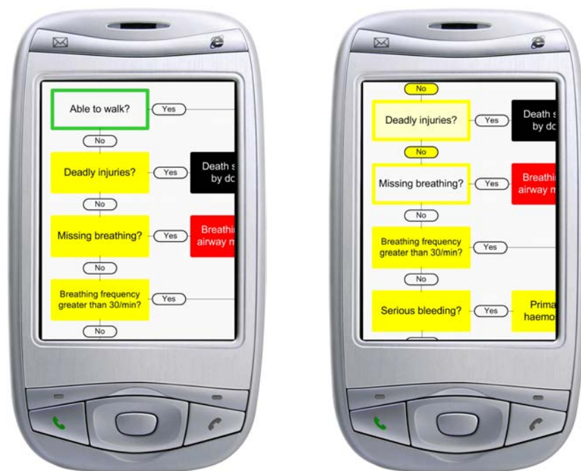
Figure 2: Information presentation in 2D. (a) Checking the patient's ability to walk on the 2D user-interface (b) Visualization of current steps and triage history
